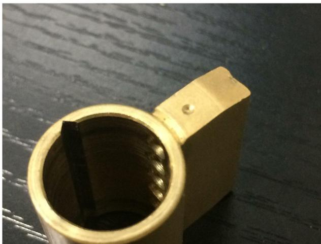
In addition to the many other features that are intended to reduce the effects of wear on both the key and lock, the dimple on the front of the plug is slightly elongated to make inserting the key easier and to reduce wear against the warding:
