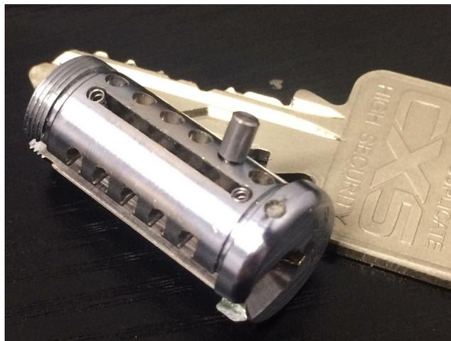
An ASSA gin bottle pin stuck in the construction keying holes
