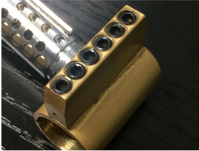
Set screws plugging the pin chambers
