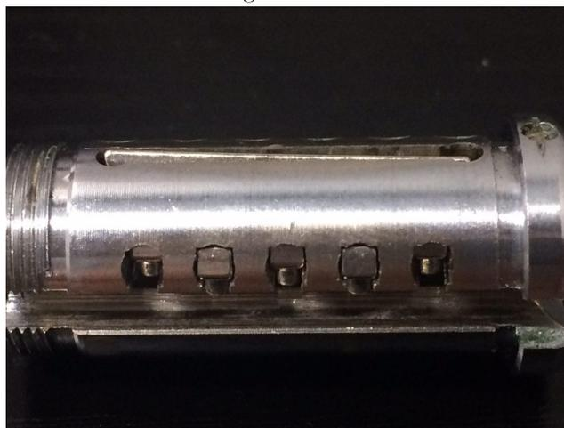
Above is a picture of a sidebar where the front three sliders are set to true gates while the rear two are set to false gates. Note the angle the sidebar is allowed to engage the sliders. This is plenty to allow the lock to open with little resistance.
