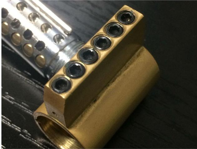
Set screws plugging the pin chambers
