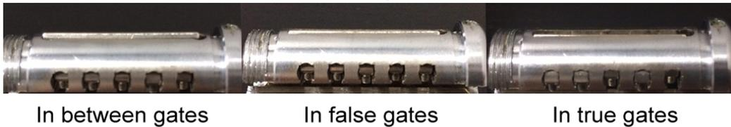
Making this easier is the fact the sidebar has nothing forcing it to remain parallel with the plug, as many other sidebar designs do and this allows the sidebar to rotate a bit and enter the plug at an angle, using some true gates and some false. By using ridges between the side pin chambers, the sidebar has much less room to do this.
