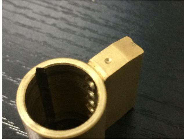
In addition to the many other features that are intended to reduce the effects of wear on both the key and lock, the dimple on the front of the plug is slightly elongated to make inserting the key easier and to reduce wear against the warding:
