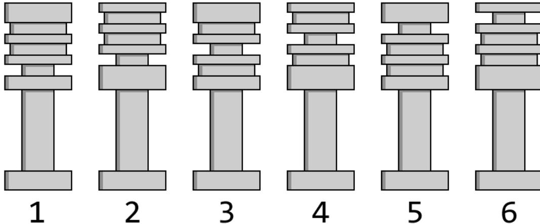
Scale drawing of all six cuts of pin
