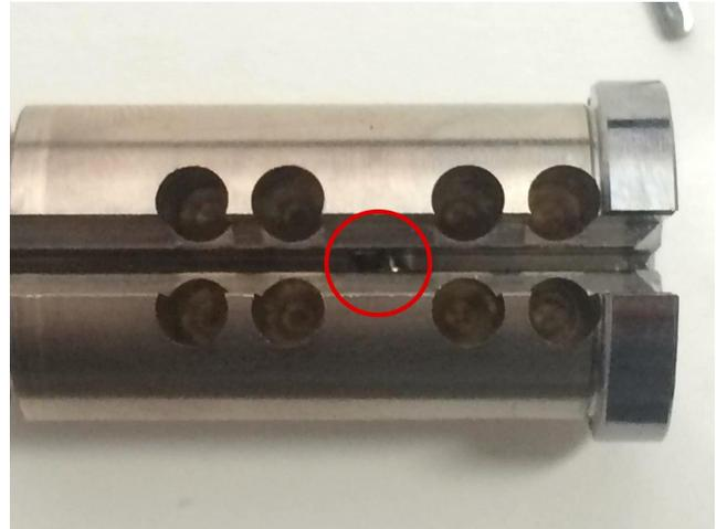
Key retention pins in place within the plug
