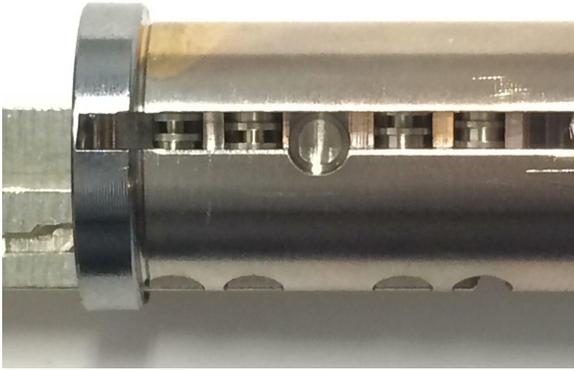
View down the sidebar slot. Side pins misaligned.
