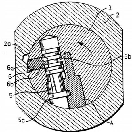
Sidebar cam action from the Desmo patent (US5517840A). Note the sidebar (6) and slot (2a).
