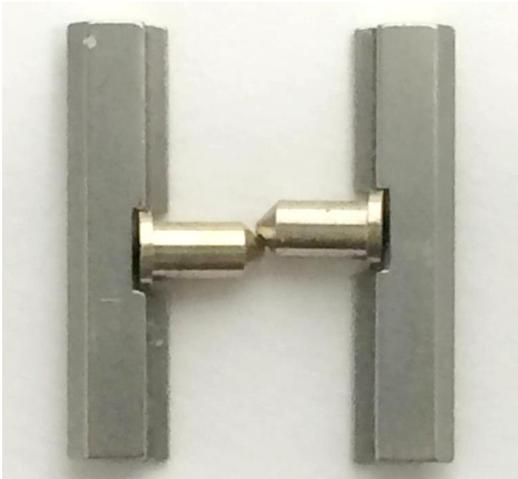
Key retention pins as they engage with the sidebar. Note how the spacing with one in front of the other allows them to touch.
