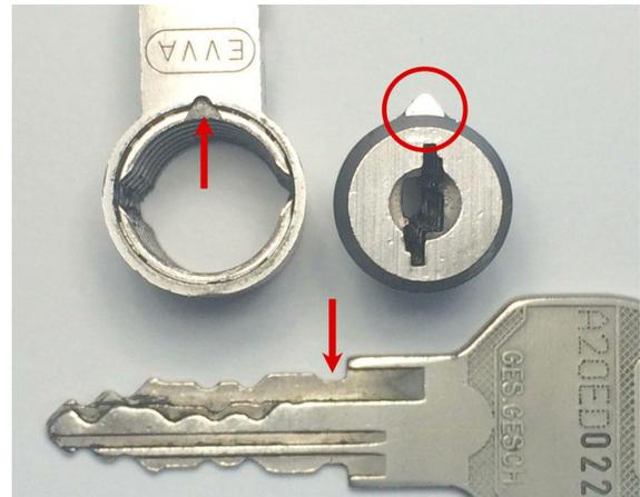
EVVA Dual key retention bar. Arrows show where it releases into the housing and grips the key.
