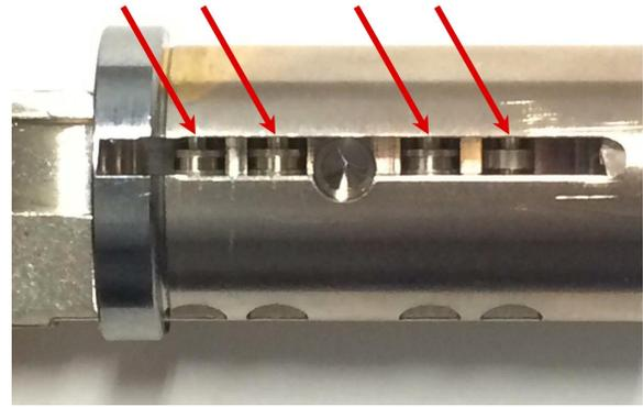
Same view, side pins correctly aligned. Note how the gates align at the very top of the slot to match the sidebar fence.
