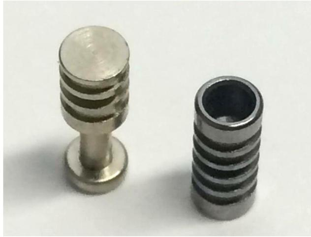
Top of Desmo pin compared to top of Twin 6000 side pin
