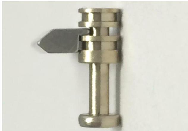
Close up of sidebar engaging with true gate on a 4-cut pin
